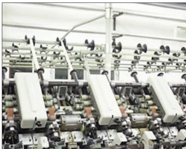
Fig. 1. Production of vortex yarns on MVS 810 spinning machine
