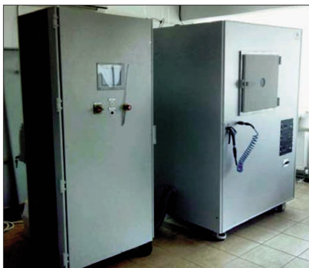
Fig. 1. Gas plasma CD400 Roll-to-roll installation
