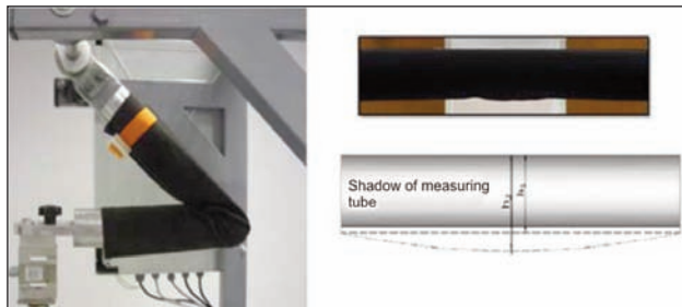
Fig. 2. Test process, deformed fabric sample by artificial human elbow and measurement of bagging deformation on a measuring tube
